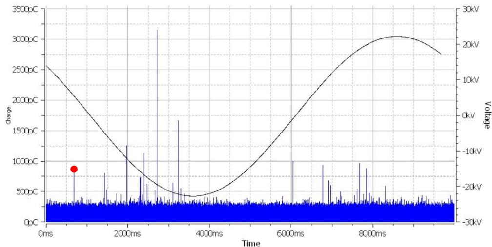
Figure 4. PDIV Graph of Partial Discharge Testing
