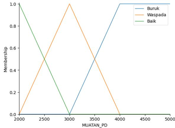
**Figure 12. PD Charge Membership Function**
