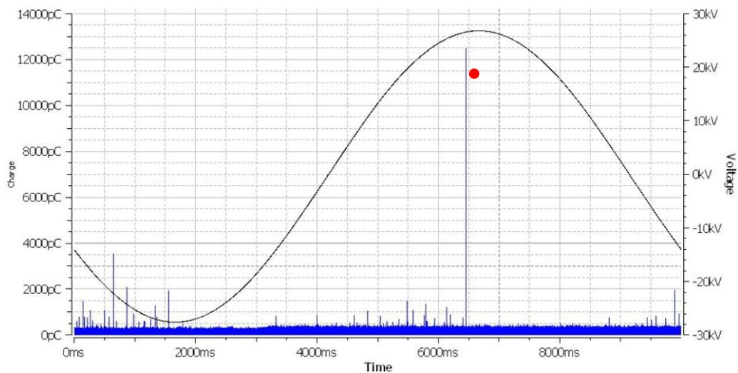
Figure 5. PDEV Graph of Partial Discharge Testing
