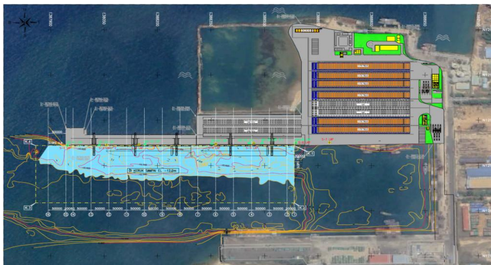
Figure 2. Dredging Layout on Existing Piers
