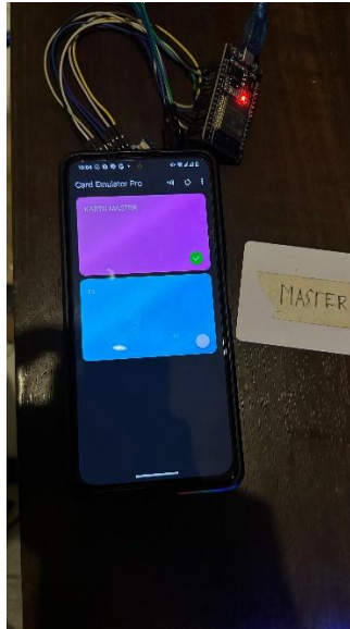
Picture 9. Bringing an android smartphone closer to the RFID-RC522
