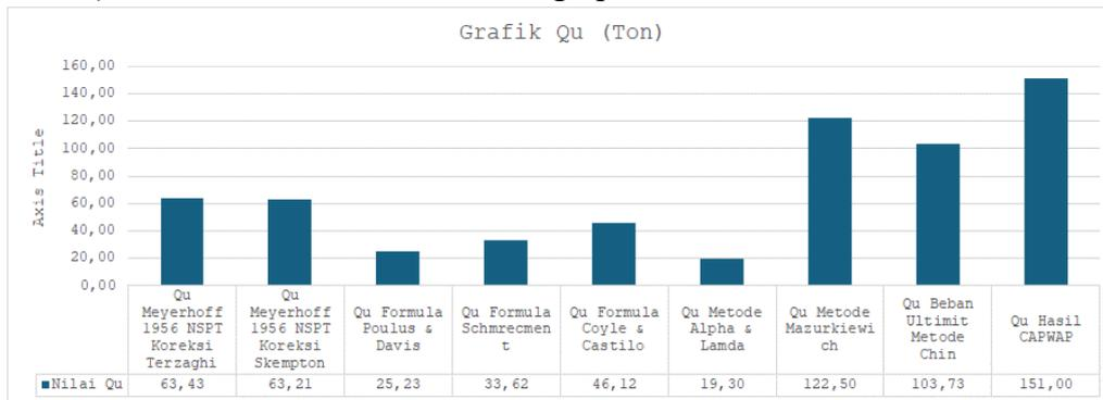
Figure 14. Qu values from the calculation using the Static formula Meyerhoff (1956) NSPT Terzaghi and Skemton, Poulus & Davis, Schmrecment, Coyle & Castilo, as well as the Alpha & Lamda Method and the Static (Mazurkiewich & Chin) and Dynamic (CAPWAP) Test Results
