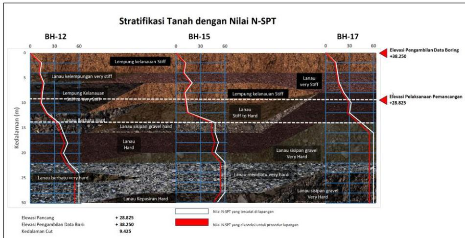
**Figure 6. Soil Stratification Drawing, N-SPT Value and N-SPT Value corrected according to Skempton**
