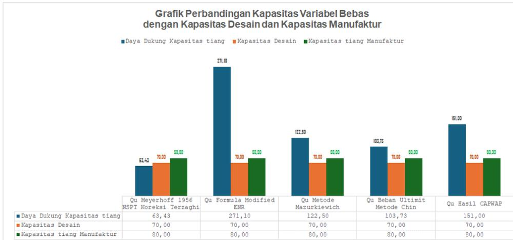
Figure 17. Comparison Chart of Free Variable Capacity with Design Capacity and Manufacturing Capacity
