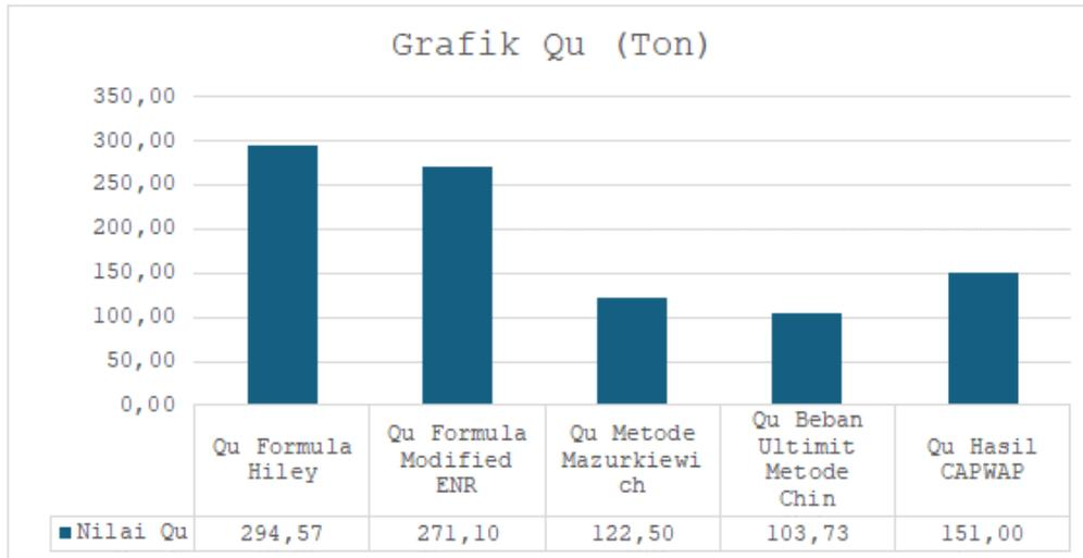
Figure 15. Qu values of the calculation results using the modified Hiley and ENR dynamic formulas and Static (Mazurkiewich & Chin) and Dynamic (CAPWAP) Test Results
